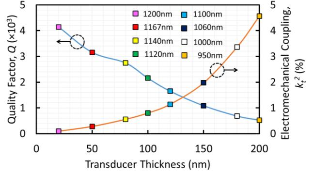
Figure 3: Simulated performance metrics (quality factor,  $Q$  on left Y-axis and electromechanical coupling,  $k_r^2$  on right Y-axis) for 8 GHz FoS-FinBARs created from different combinations of HZO transducer thickness and fin width.
