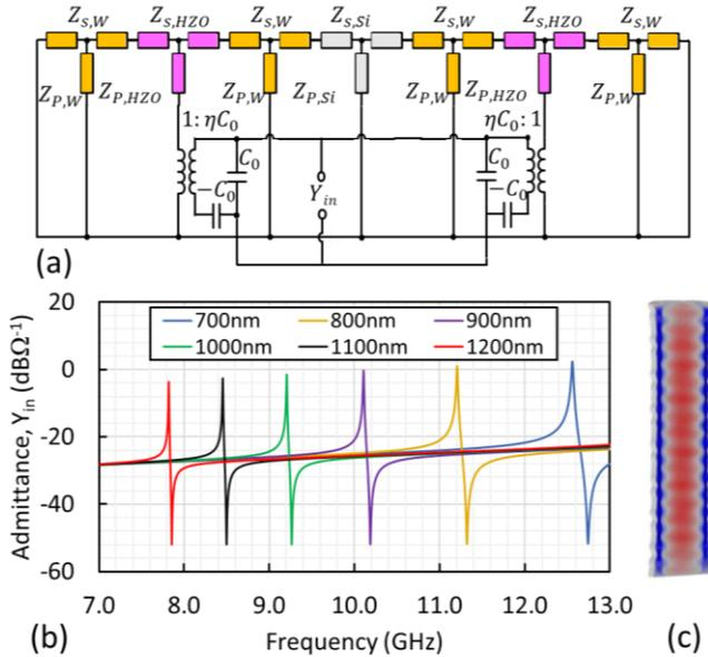
Figure 2: (a) Electrical equivalent circuit model from Mason's waveguide approach for FoS-FinBAR; (b) simulated admittance of FoS-FinBARs with different fin widths, operating in 3<sup>rd</sup> width-extensional bulk acoustic mode ( $WE_3$ ), highlighting lithographical frequency scalability; (c) COMSOL simulated cross-sectional mode-shape of FoS-FinBAR operating in  $WE_3$  mode.
