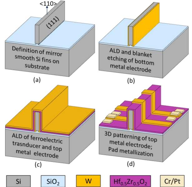
Figure 4: Three mask fabrication process flow of FoS-FinBARs: (a) wet-etching Si fins with (111)-plan etch-stop; (b) ALD and selective patterning of the first W electrode; (c) ALD of ferroelectric HZO transducer and top metal followed by crystallization annealing; (d) 3D patterning of top gates by isotropic dry etch.
